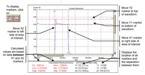
You can also zoom in on a specific area of the waveform. Zooming in only rescales the display, no calculations are performed in the zoom area.
