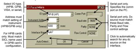
If there seems to be no communication between the Agilent 14565A application and the dc source, select **Auto Detect** to detect any dc sources connected to your pc. Also, try resetting the I/O interface by clicking the red reset button. This also resets the dc source to its default settings.
