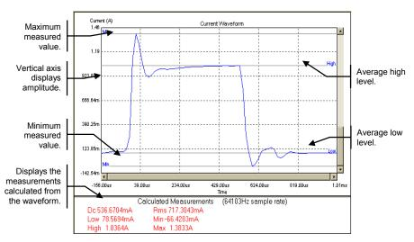
The values in the measurement area at the bottom of the display are calculated from the all of the data that is captured in the display. If horizontal markers have been set, measurements are calculated only from the data between the markers. Refer to Performing Measurements on Waveforms.
